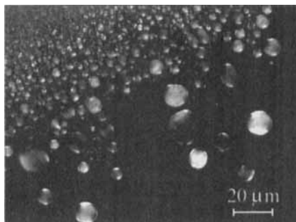
FIGURE 3 Optical micrograph showing the typical PDLC morphology outside the laser-spot area. The dimension of the liquid crystal droplets increases on moving away from this area.
